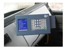
When the loading or unloading is complete, he will press a key to allow the system to process the weighment, complete the transaction and print the tickets. A re-print button is provided in case the driver needs an additional copy.
