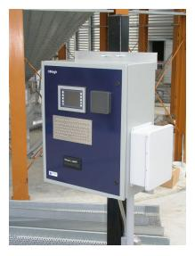
An 80 mm wide thermal ticket printer is installed to provide drivers with multiple transaction tickets for the driver as well as the crop owner. Duplicate transaction tickets can also be printed to any other standard laser printer(s) located on the Dawson Farms network.
