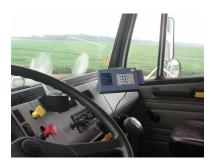
The password protected data is maintained in memory until it is changed again so that the driver can deliver multiple loads so as long as the crop or location information does not change. When the driver pulls on to the scale, the terminal automatically connects to the wireless network, to transfer his load information he simply presses the F1 (*Scale*) key.
