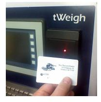
The driver simply presents the card within 4" of the gray reader to the right of the screen, and all the transaction data is displayed for his approval on the screen. A network based software utility is used to preprogram the cards by number from the office, with a pre-selected set of load parameters including Crop, Farm, Bin, Truck #, Etc.
